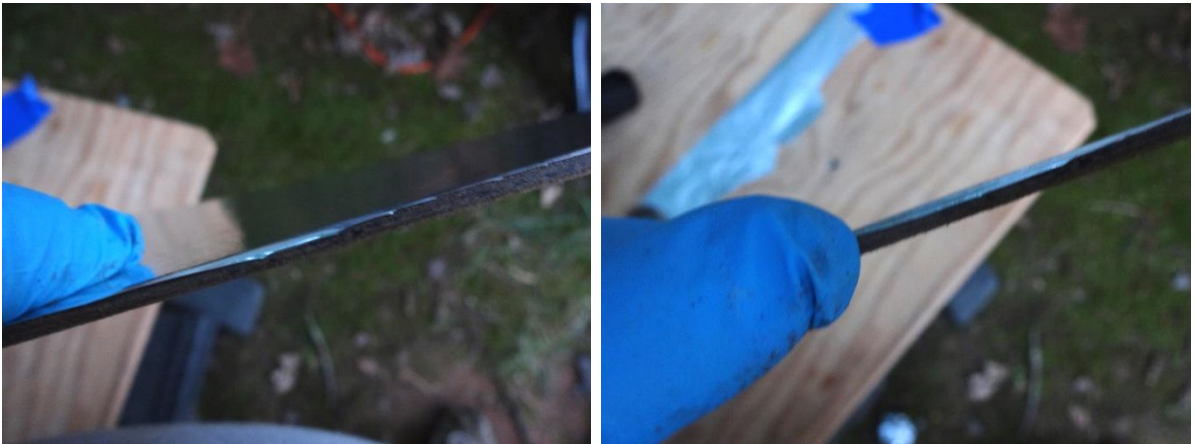
Before and after rolling and burnishing:
