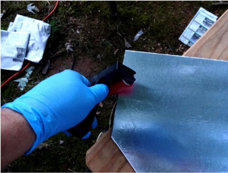
Before and after rolling and burnishing:
