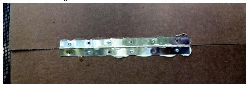
10. Here you see the alternating the screws in the holes in the hinges:
