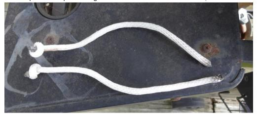
14. Thread the rope through the hole that is ¾" from the edge from white side to brown, with the knot on the white side
